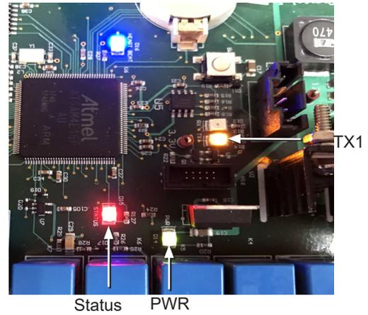
**Figure 35: Application Loaded but no Bootloader**
