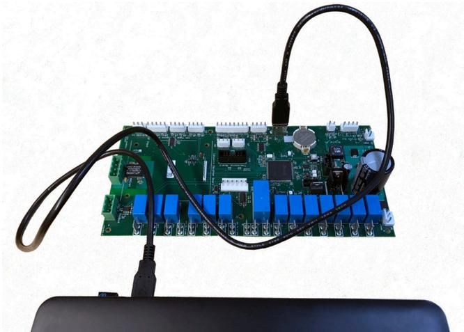
**Connecting a USB-C Device to the MicroTech Controller**
